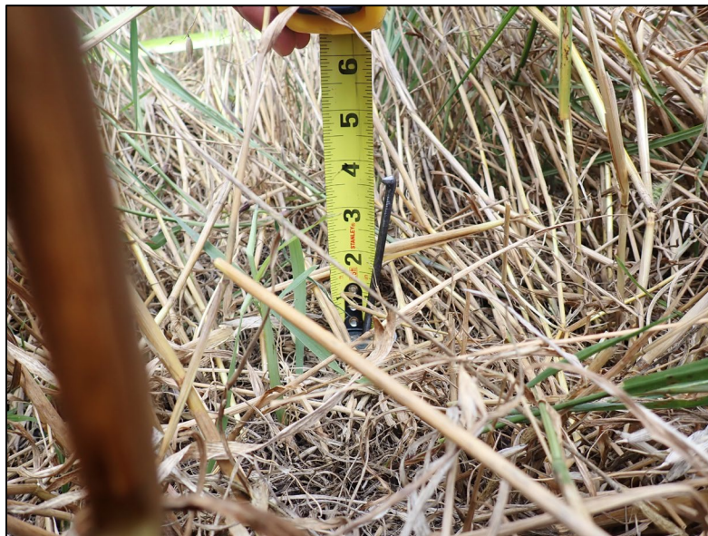
Picture 6. Erosion pins that were deployed within our experimental plots to assess seed mixture erosion prevention.
