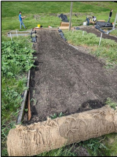
Picture 4. Seeded vertical stripe on experimental levee prior to jute cloth application.
