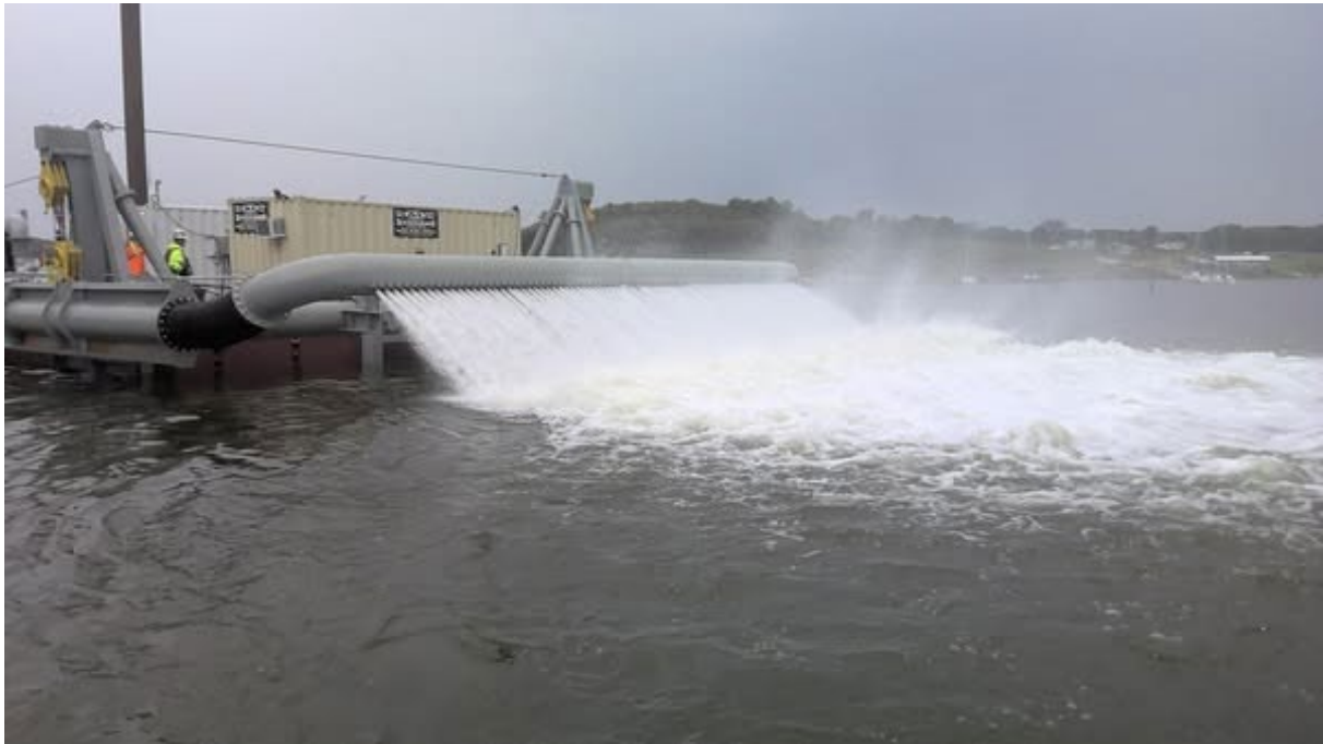
Picture 2. Tuttle Creek water injection dredge (WID) demonstration. (Top) Fully assembled WID in Tuttle Creek Reservoir (Photo credit Laura Totten). (Bottom) Water jetting from WID spray bar (Photo credit Laura Totten).
